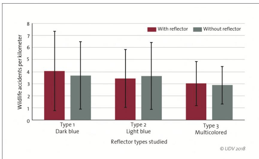
Fig 7 Number of wildlife accidents per kilometer and year on test stretches of road with the three optical wildlife warning reflectors tested
