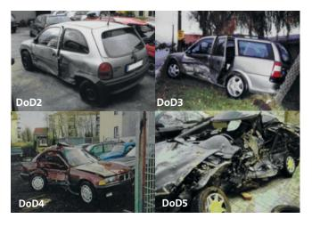
Figure. 1: Examples for Degree of Damage (DoD) according to German Insurers Accident Research definition
