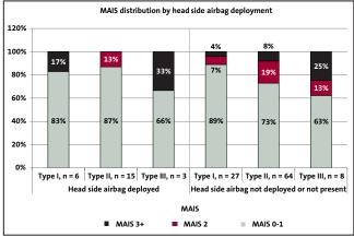
Figure 8: MAIS distribution for cars with deployed and non-deployed head side airbags (models 1997 and later)
