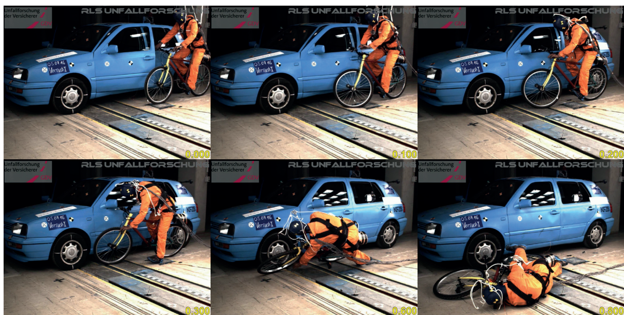
Figure 14: Collision with a driver's door open at an angle of 26.5 degrees and with a small overlap in the handle area of the handlebar
