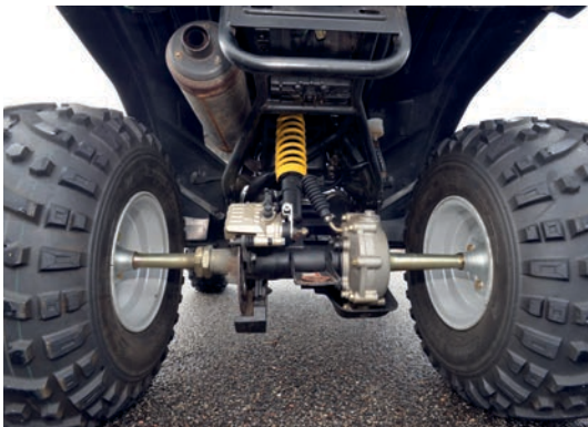
Figure 2: Quad bike without differential
