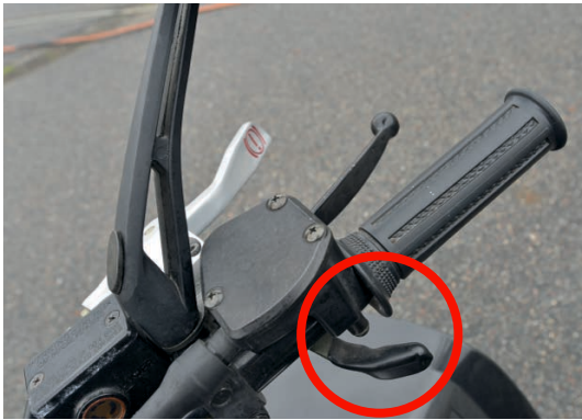
Figure 1: Quad bike with thumb throttle
